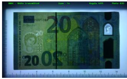
Comparison between the examined banknote in white transmitted light with the reference banknote from the database
