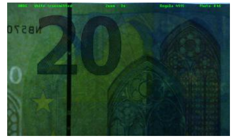
Fragment of the examined banknote in white transmitted light. 2x magnification on the monitor
