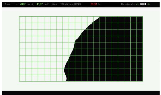
Automatic measurement of the banknote area (residual area)
