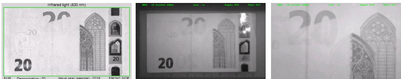
Comparison between the examined banknote in infrared incident light (830 nm) with the reference banknote from the database
