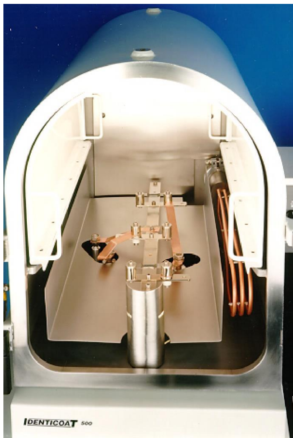
View inside the Identicoat 500 chamber showing the evaporation sources and shields
