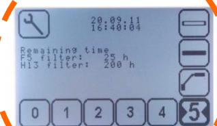
The touch panel display also informs the user about a due filter replacement for the pre-filter mat or the fine particulate filter cassette.
