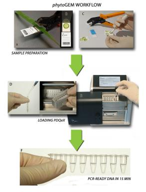
**Figure 1:** The steps for plant DNA extraction using the *phyto*GEM system. Leaf samples are crushed using the *phyto*GEM crusher tool (A) onto storage cards (B). Circular punches are taken (C) and transferred into PDQeX tubes (D). Tubes with punches and reagents are inserted into the PDQeX (E) and run through an extraction program. High quality, clear plant DNA (F) is ready for downstream applications.
