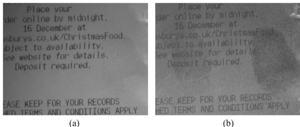
Fig. 2. Detection of latent fingerprints on thermal paper by (a) longwave UV-A and (b) shortwave UV-C.
