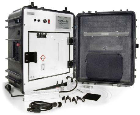
The Cyanoacrylate fuming chamber, now available with **touch panel**, is a good method to secure evidence for all items with non-absorbent surface.
