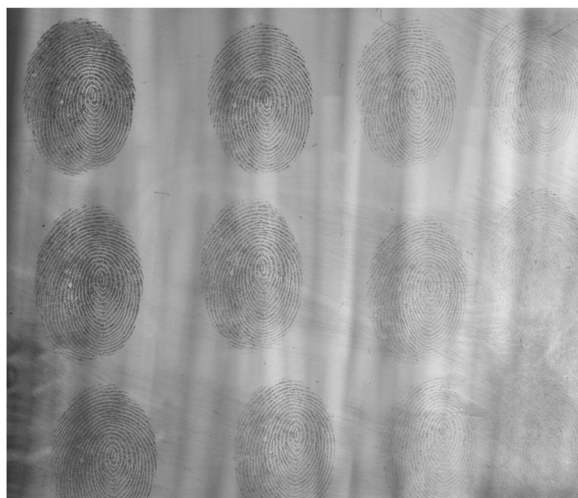
Fig. 10. Depletion series of natural fingerprints deposited on a glass substrate and imaged using UVC reflection after 1 day.
